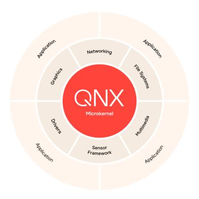
The QNX microkernel architecture isolates components that are not safety-critical from those that are, streamlining system certification processes.
